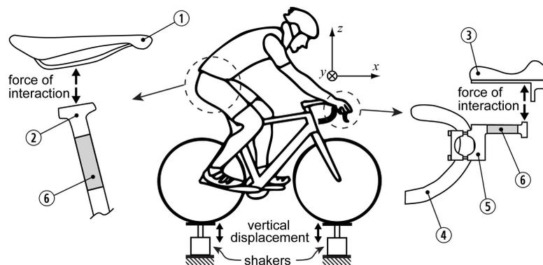
Fig. 2. Road simulator equipped with two shakers for bicycle vibrational transmissibility assessment. The bicycle is equipped with an instrumented seat post and two instrumented brake hoods. 1-saddle; 2-seat post; 3-hand rest; 4-handlebar; 5-brake hood body; 6-strain gauges area.
