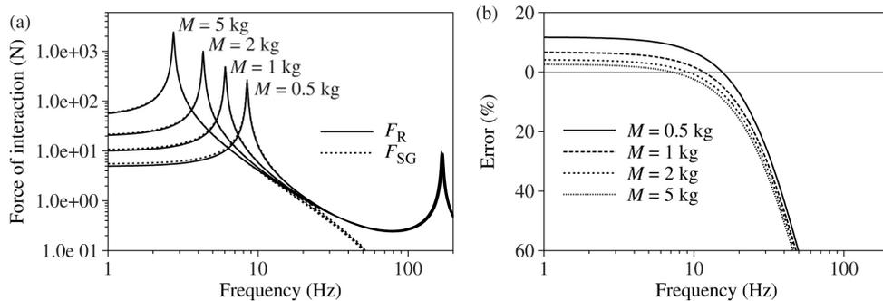
Fig. 4. Force of interaction (a) and measurement error (b) for the simple beam transducer with suspended mass values of 0.5, 1, 2 and 5 kg.
