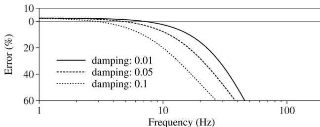
Fig. 6. Measurement error for the simple beam transducer with suspended mass of 5 kg for modal damping ratio values of 0.01, 0.05 and 0.1.
