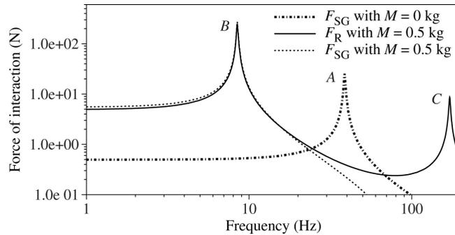
Fig. 3. Force of interaction for the simple beam transducer with suspended mass values of 0 and 0.5 kg.
