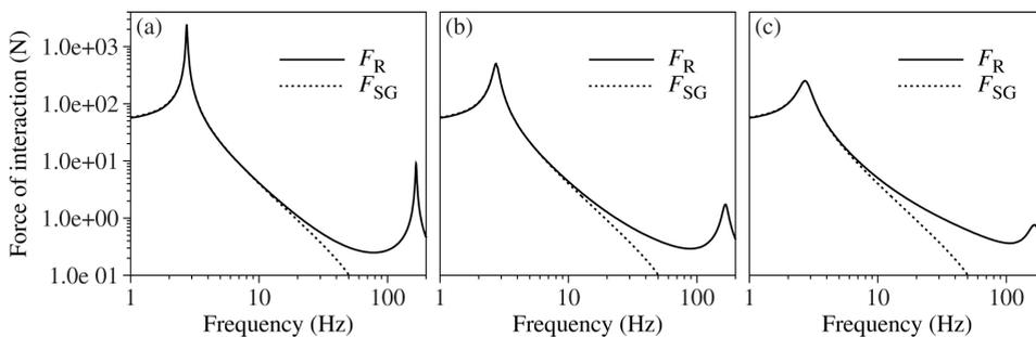
Fig. 5. Force of interaction for the simple beam transducer with suspended mass of 5 kg for modal damping ratio values of (a) 0.01, (b) 0.05 and (c) 0.1.
