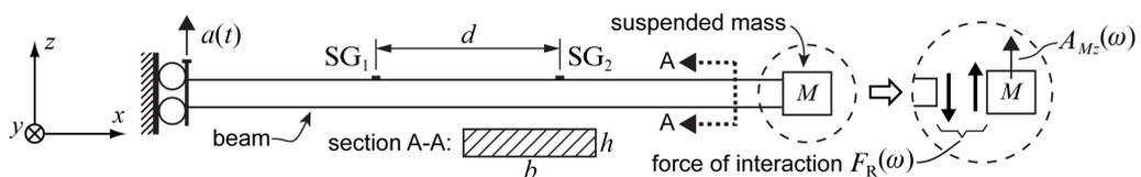
Fig. 1. Simple beam transducer model and boundary conditions. The detailed view (inside the dotted circle) shows (1) the force of interaction between the beam and the suspended mass ( $M$ ); (2) the magnitude of the acceleration of the suspended mass along the  $z$ -axis,  $A_{Mz}(\omega)$ .
