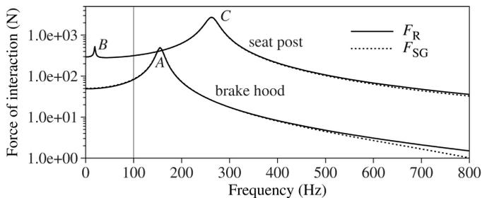
Fig. 7. Force of interaction for the instrumented seat post and brake hood (frequency range: 0 to 800 Hz). The vertical line at 100 Hz corresponds to the upper limit of the operational frequency range of these transducers when they are used for bicycle vibrational transmissibility assessment.
